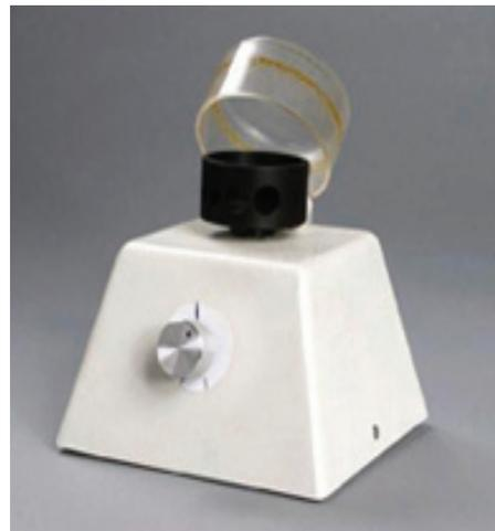
FIGURE 4 Fist prototype of centrifuge wax remover with hub rotor and ring of expelled wax from numerous tests.
